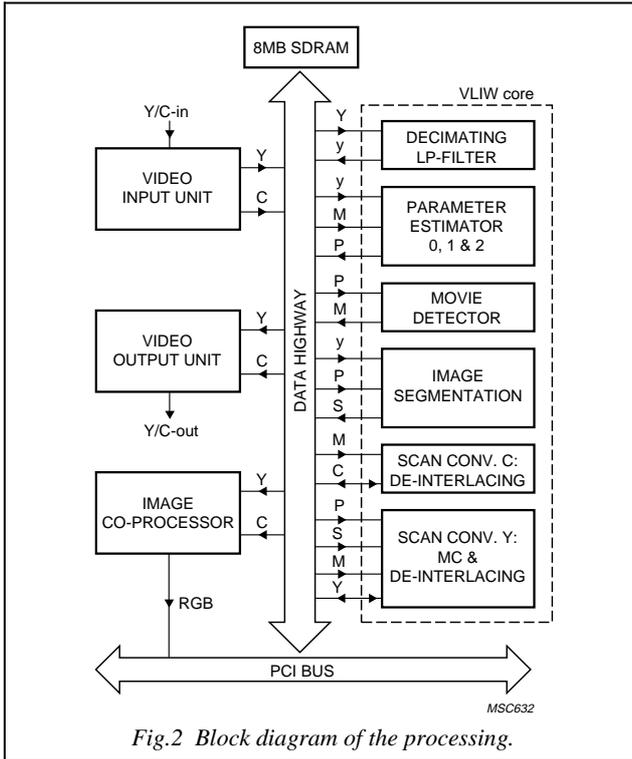
Fig.2 Block diagram of the processing.
